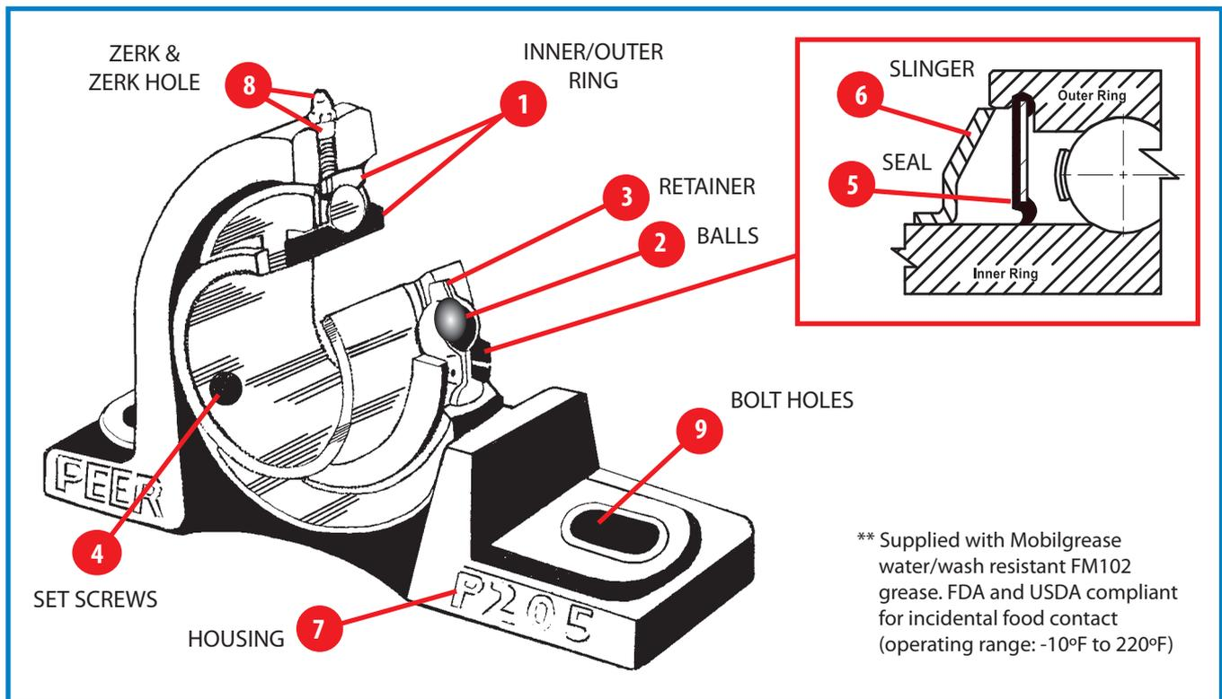
\*\* Supplied with Mobilgrease water/wash resistant FM102 grease. FDA and USDA compliant for incidental food contact (operating range: -10°F to 220°F)
